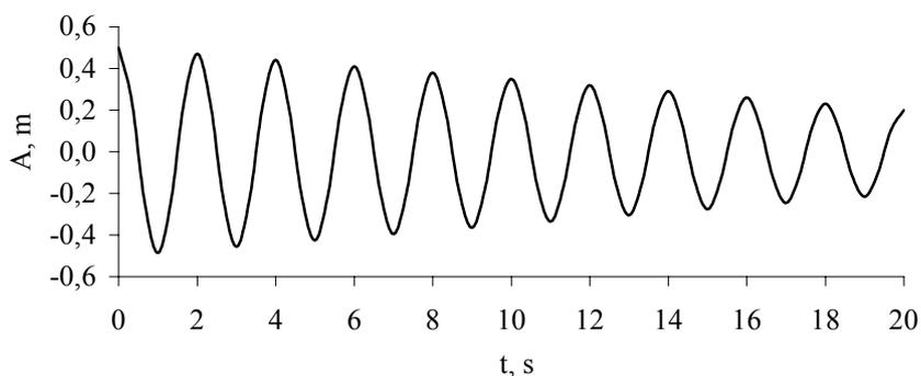
Fig. 1. Variation of amplitude (A) of pendulum deviation from the balance point with time (t)
